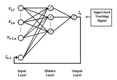
Figure 3: A typical temporal sensitive model, in this case, an out-to-input feedback model with slow learning. Inputs may include patterns over time and feedback from the prior output.  $x_{t,n}$  are the inputs from time t, and  $z_t$  is the output from time t.
