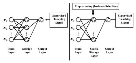
Figure 2: (left) A typical fast learning model. The storage layer replaces the hidden layer from slow learning. Each storage node is independent of each other. The Gaussian symbol represents a common non-linear distance kernel. See text for details (right) A typical maximum margin model, which extends the fast learning model. The preprocessing step limits the number of nodes in the sparse storage layer.
